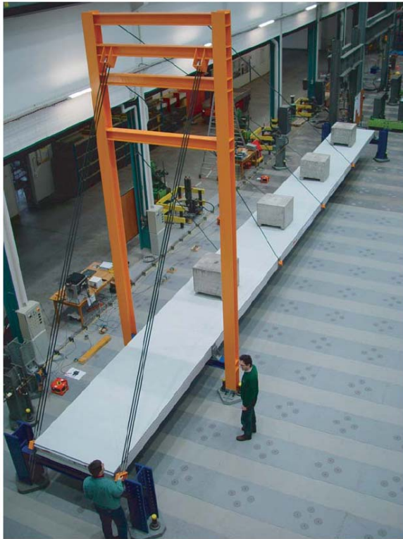
Figure 3. Laboratory test field "Adaptive cable-stayed bridge" at EMPA
