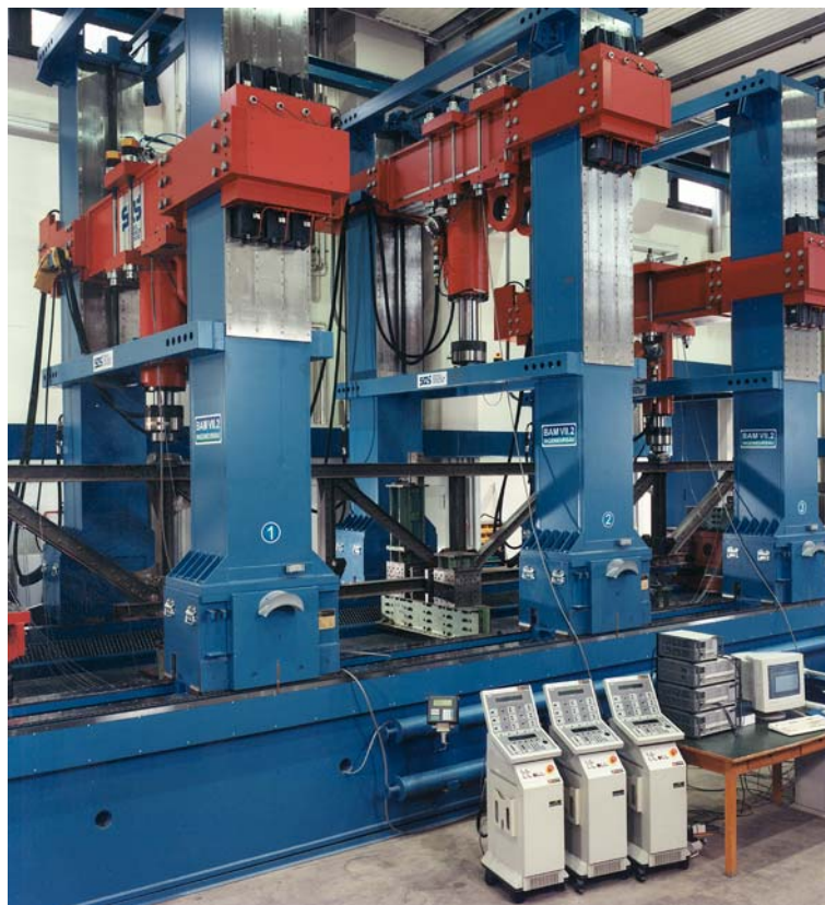
Figure 4. Universal test machine for static and dynamic loading of bridge girders at BAM
